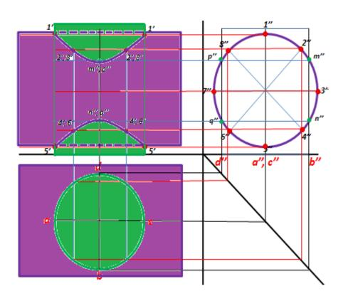
For plotting an accurate curve, certain *critical* or key points, at which the curve changes direction, must also be located. These are the points at which outermost or extreme lines of each cylinder pierce the surface of the other cylinder.
